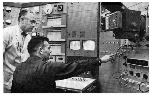
CONTROL CONSOLE of the Sandia Pulsed Reactor Facility provides for five different modes of operation of the fast burst reactor. Closed circuit television gives two views of the reactor and experiments which are conducted inside a shielded concrete hemisphere. At the console are Jennings Conant, left, and John Snyder of Reactor Division.
